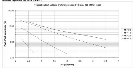
Minimal voltage for 5 m/s circumferential speed, module 2 gear, 1 mm air gap and 10 kOhm load resistance: 1.8 Vpp
